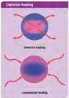
Dielectric heating works across the entire profile of the wood, while conventional heat has to be conducted into the wood from the surface.
