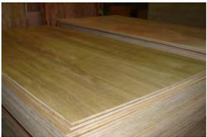
Processed WPM such as Plywood, Particle Board, Oriented Strand Board, Veneer
