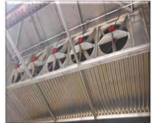
Fans should be used to maximize air flow through the wood stack
